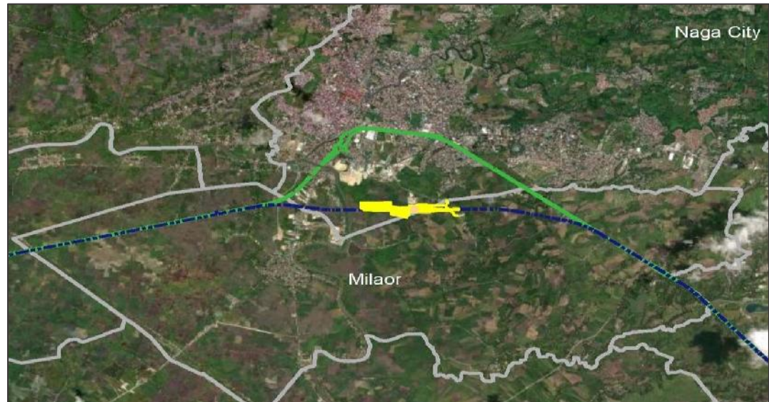
Fig. 1.19. The proposed new PNR alignment. The green line is the existing alignment, while the dark blue line represents the new alignment. The yellow portion represents the new station.
